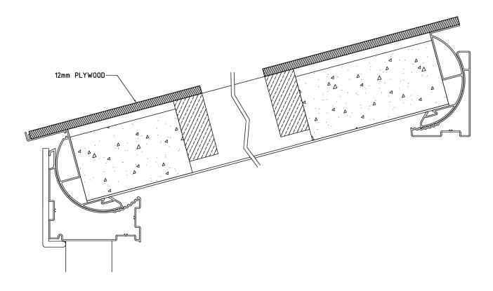
8. Once eaves guards have been installed to around the 18mm OSB decking, install the roof felt overlapping onto the 47x125 timber and 12mm Plywood.
