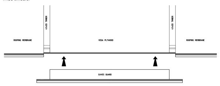
10. Run a continuous bead of sealant all the way down the edge of the roof deck where the Vega glazing panel will overlap. Then position the Vega glazing bar to extend 30mm past the eaves guard, then fix down the central channel into the 95x125mm timber using 4.2x38LG screws at 300mm centres.
