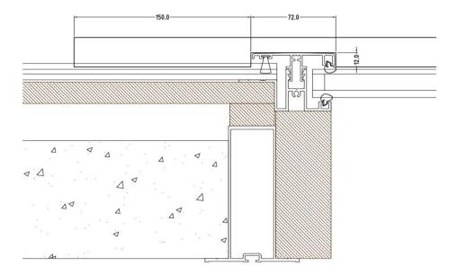
2. Screw ventilator strips to the batten using 4.2x16LG screw to the 25x38mm batten. Apply expanding foam tape to the underneath of the batten where it spans across the glass and then position so the outside edges of the ventilation strips will suit the inner width of the Slateskin ridge. . Screw the timber down to the roof deck at both ends using 2 x 60mm baypole screws. (Do not use baypole fixing directly above the glass)
